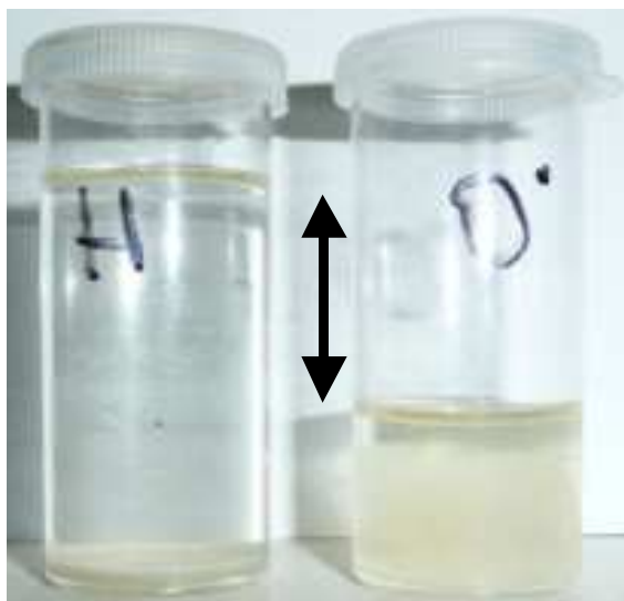
Figure 3. There is a swelling of starch in water ( \sim 20^\circ\text{C} ) with a different electric potential. Starch for months does not swell in water with a potential of -250\text{ mV} (left), but swells in water with a potential of +250\text{ mV} in a few minutes (right). The electric potentials of electrified waters were measured relative to uncharged water.
